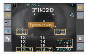
The pachymetry data can be used to display a corrected IOP value.
