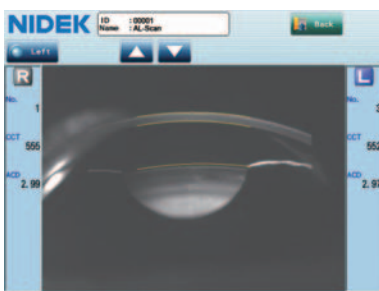
Sectional lens image (Scheimpflug image)
